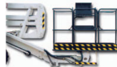
⑤ 180° hydraulic rotating system.
