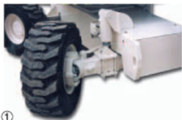
① Traction system with differential groups and oscillating shaft incorporated in one of them.
